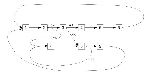
The product units are mounted on pallets as they enter the system at station 1. Finished products are dismounted from the pallet behind station 6. The throughput of station 6 is hence equal to the throughput of the system in terms of completed product units. Transportation times as well as the times required for the mounting and dismounting processes are negligible.
